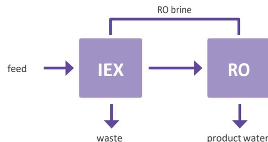
This technique is economically viable if the RO concentrate is recirculated for the regeneration process. Promising results were also obtained for other water types (e.g. treated wastewater). This indicates that the technique is widely applicable.
